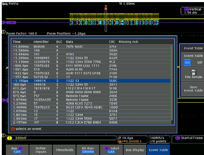
Event table showing decoded identifier, DLC, DATA, and CRC for every CAN packet in a long acquisition.
